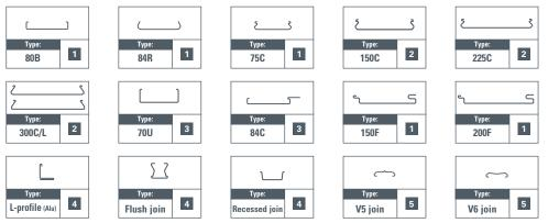
Flush-, V5- and V6 join profile only for 84R. Recessed join profile only for 80B.
